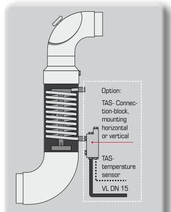
Vertical or diagonal on a heat source with 2 x 90° flue pipes and large cleaning door cleaning door as S-shaped surface-mounted variant
